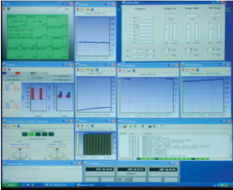
The MAIB VDR readout facilities allow inspection of technical parameters as well as sound from the bridge, and radar data.
